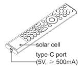
You can charge the remote by exposing the solar cell to light or using a USB type-C cable(not provided).
