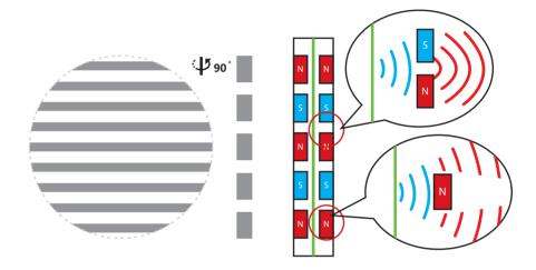
Unlike the sound waves created by a conventional magnet, the special shape of stealth magnet of SUSVARA enables the waves to pass through the magnet without generating interference.
