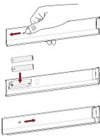
1. Slide the back cover to open the battery compartment of the remote control.
