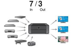
This unit is equipped with 7 HDMI inputs enabling connection to various HDMI compatible devices such as Blu-ray Disc players, game consoles and HD video camcorders. There are dual HDMI outputs for the main room, and a third HDMI output for another room.
