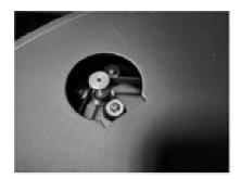
1. Install the drive belt over the inner ring under the platter and make sure it won't fall off during the setup.
