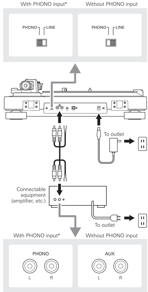
\* Depending on the equipment you are connecting, a ground (earth) terminal may exist near the phono input jack. If this is the case, connect to it using the ground line from the RCA audio cable. This will help prevent a low humming noise that might otherwise be heard during playback.
