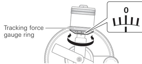
2. Turn the counterweight and the tracking force gauge ring together counterclockwise (to the left) until the centerline value matches the recommended tracking force value for the cartridge you are using.
