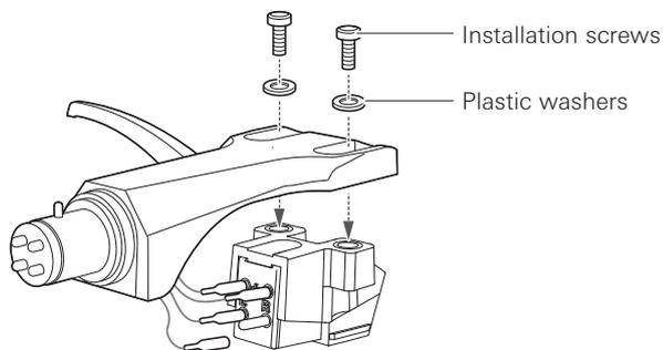
6. **Using a commercially sold, non-metallic slotted screwdriver, tighten the screws in both places, and then adjust the overhang.**
