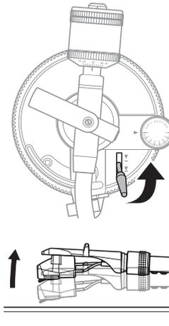
3. Position the tonearm over the desired location (groove) on the record.
