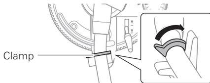
3. While still lightly holding the headshell, turn the counterweight to adjust the tonearm's balance.
