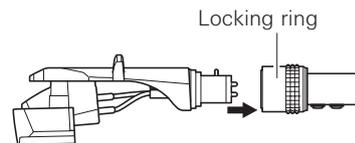
3. With the headshell inserted, turn the locking ring counterclockwise (to the left).
