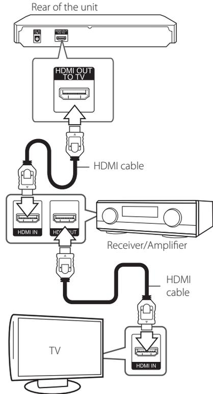
Connect the amplifier's HDMI output jack to HDMI input jack on your TV using a HDMI cable if your amplifier has HDMI output jack (Refer to amplifier's owner's manual).
