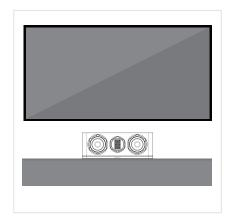
The centre channel loudspeaker should be positioned centrally between the loudspeakers, close to the television and mounted above or below the screen.
