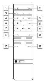
If the remote control will not function, please check that the batteries have not expired, and that there is nothing blocking the front panel IR sensor, which is located in the EVO 75/150. There is no IR sensor located in the EVO CD.
