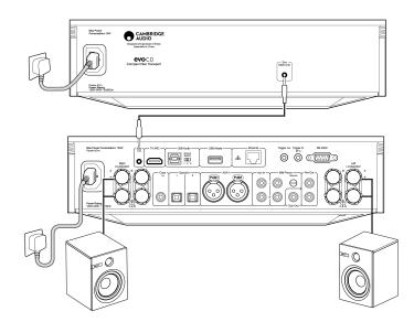
**Note**: We do not recommend placing the EVO CD right next to and touching your EVO 75/150, if you are placing the units side by side. The EVO 75/150 Wi-Fi and Bluetooth antennas are located in the sides of the unit, and another device touching this can reduce Wi-Fi and Bluetooth signal strength and effect connectivity.
