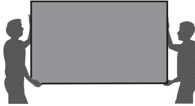
2. Place the assembled screen vertically on the ground. Look at the screen horizontally, and if you find the material is black, it is in the correct direction and ready for mounting on the wall. However, if the material is white, turn around the screen and then install it.
