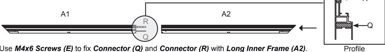
3) Use **M4x6 Screws (E)** to fix **Connector (Q)** and **Connector (R)** with **Long Inner Frame (A2)**.
