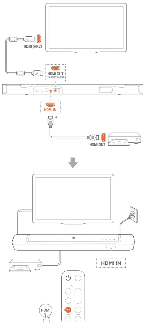
1. Connect the soundbar with the HDMI IN (ARC) connector on your TV by using the supplied HDMI cable.
