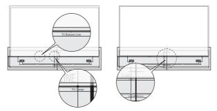
3 With a pen, mark screw holes on the installation guide where the wall brackets will be attached.
