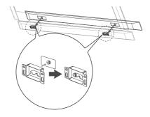
8 Fix the hooks of the unit on the brackets as shown below.
