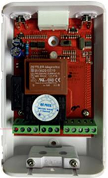
**Central control wiring** The interface adopts 6P crystal head wiring **Contact control** Weak current relay
