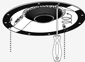
Push speaker into hole and tighten all 3 Tri-Grip Dog Legs
