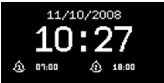
The **Standby screen** shows the time, date and any active alarm times.
