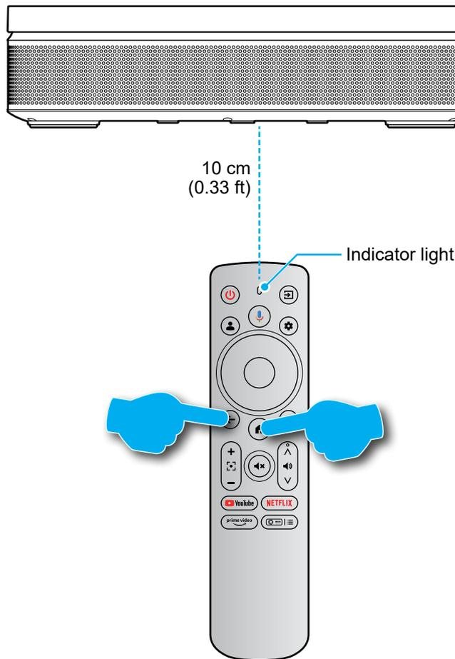
3. When you see pairing successful message on screen, this indicates the remote control is successfully paired.
