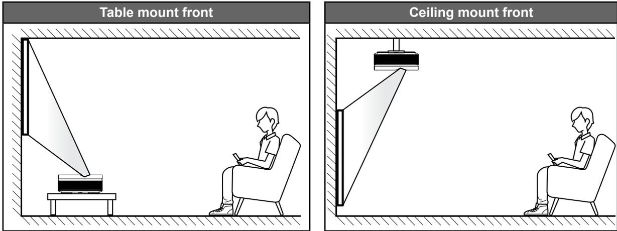
Projector should be placed flat on a surface and 90 degrees / perpendicular to the screen.
