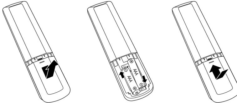
**Note:** Replace only with the same or equivalent type batteries.
