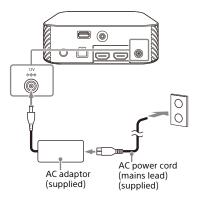
2 Connect the AC power cords (mains leads) (supplied) to the AC inlets on four speakers, then connect to the AC outlets (mains).
