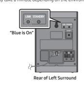
. If the LINK LED does not turn to solid blue in a minute please repeat from step 2 through 5 referring to step 6
