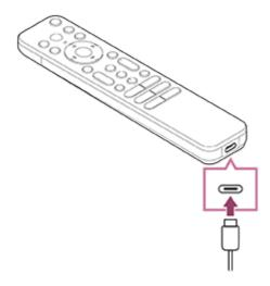
Connect the USB cable to your USB mains adaptor.The LED above the microphone lights up red when charging starts.
