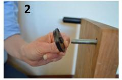
Slide the isolation disc down the bolt making sure the protruding lip located on the inner hole is facing the wood
