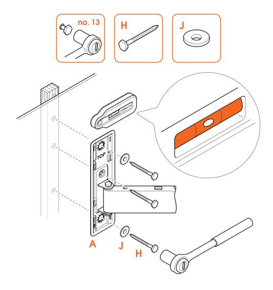
5. Attach the **wall mount** (A) to the wooden studs with the **screws** (H) and **washers** (J). Use the **spirit level** (①) to level the wall mount.
