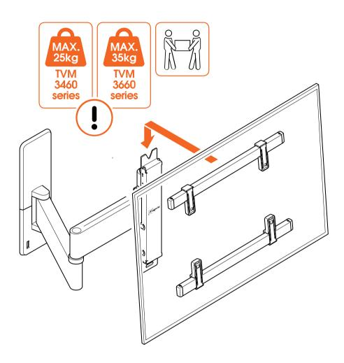
1. Carefully lift and attach the TV to the **wall mount** (a). Place the upper **interface screw** (b) in the top notch of the wall mount.
