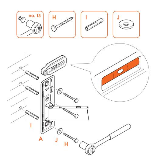
3. Attach the wall mount (A) to the wall with the screws (H), washers (J) and plugs (I). Use the spirit level (O) to level the wall mount.
