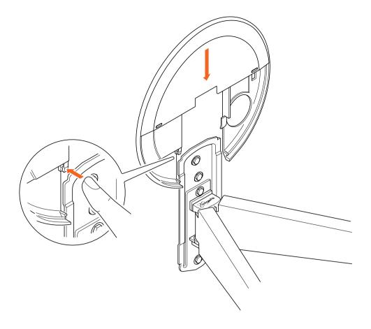
5. Slide the **upper wall plate cover** (S) onto the **wall mount** (A). To remove the cover plate, press the left tab and slide it off the wall mount.
