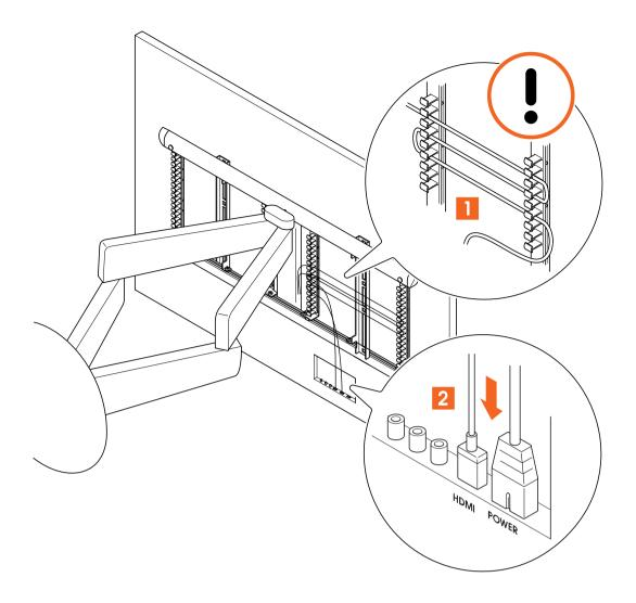
4. Connect the power cable and the other cables to the TV. Make sure all other cables are neatly stowed away by using the vertical cable clip strips on the **interface**.
