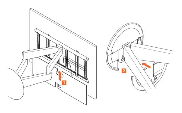
5. Put the **lower wall plate cover** ① onto the wall mount and the **interface cover** ⑨ onto the back of the **interface**.
