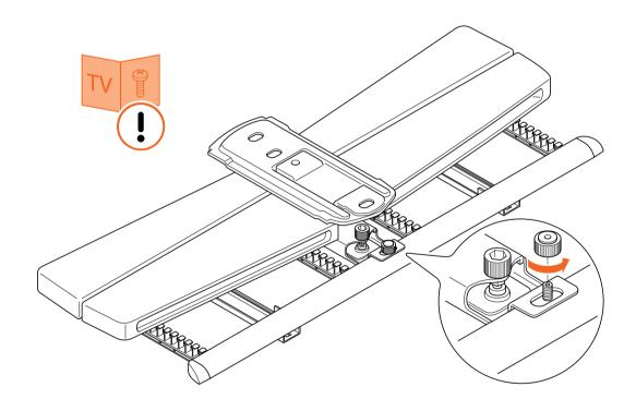
2. Remove the **thumbnut** and detach the **wall mount** (A) from the **interface**. Keep the **thumbnut** for later use.
