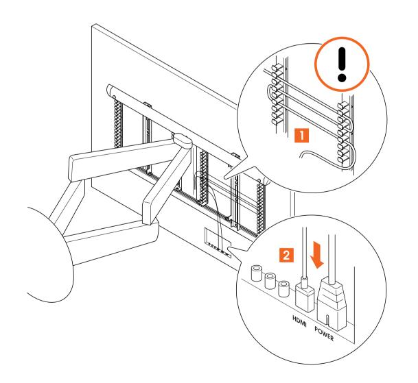
5. Connect the power cable and the **HDMI 2.0 (2 meter) cable** to the TV. Make sure all other cables are neatly stowed away by using the vertical cable clip strips on the **interface**.
