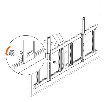
2. Secure the interface to the **wall mount** with the saved **thumbnut** from step 1.
