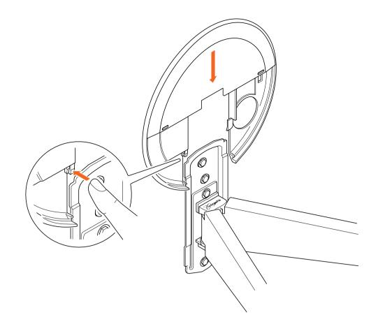
5. Slide the wall plate cover (K) onto the wall mount (A). To remove the cover plate, press the left tab and slide it off the wall mount.
