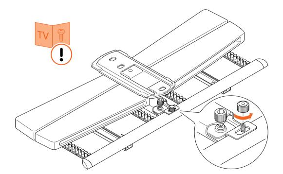
2. Remove the **thumbnut** and detach the **wall mount** (A) from the **interface**. Keep the **thumbnut** for later use.
