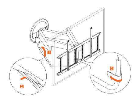
1. Attach the **cable sleeve** (1) to the **wall mount** (A), by sliding it into the holes on the bottom side of the right arm.
