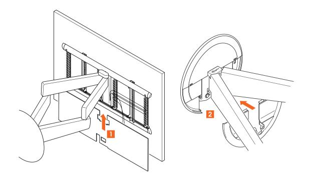
6. Put the **wall plate cover** (K) onto the wall mount and the **interface cover** (Y) onto the back of the **interface**.
