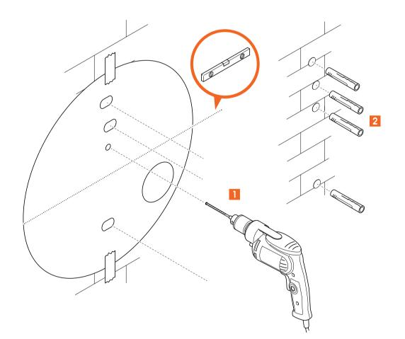
2. Drill the holes. Make sure to drill the positioning hole first. Pre-drill with a smaller drill to avoid damage to the wall.
