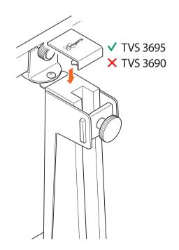
2. Apply the click-on stainless-steel **cover plate** (P) on top of the **steel bracket** (U). (TVS 3695)
