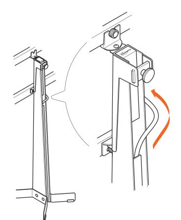
1. Carefully guide the cables through the back of the wooden / steel stand  $\mathbb{R}$ .
