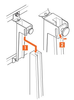
1. Slide the **steel bracket** (1) over the top of the **wooden / steel stand** (R). Use the knob (see illustration) to fasten the **steel bracket** (1) to the top of the **wooden / steel stand** (R).
