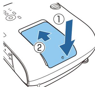
**9** Tighten the lamp cover fixing screw.
