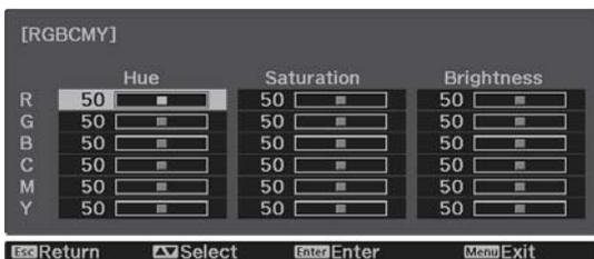
3 Use the up and down buttons to select **Hue, Saturation, or Brightness**.
