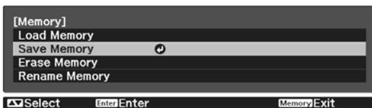
4 Use the up and down buttons to select the memory name you want to save, and then press the [Enter] button to confirm the selection.
