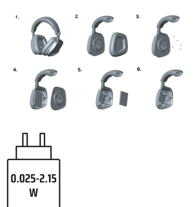
The power delivered by the charger must be between min 0.025 Watts required by the radio equipment, and max 2.15 Watts in order to achieve the maximum charging speed.
