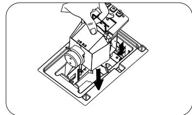
10. Tighten the screw(s) that secures the lamp.
