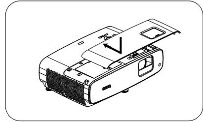
15. Tighten the screw that secures the lamp cover.
