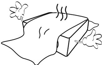
If the ventilation holes are seriously obstructed, overheating inside the projector may result in a fire.
