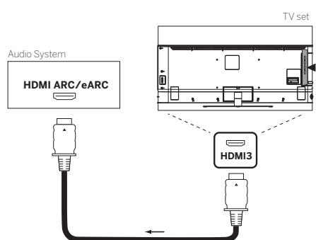
Use an HDMI cable (not supplied) to connect HDMI eARC socket of the TV set to the HDMI ARC/eARC socket of an audio system or soundbar. It is recommended to use a cable marked as „Ultra High-Speed HDMI Cable“ with a Type A connector.
