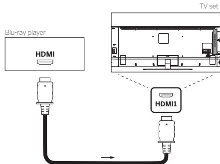
Connect the device by an HDMI cable with a Type A connector (not supplied) to one of the HDMI sockets of the TV set. To fully enjoy the capabilities of your TV, use a cable labelled „Premium High-Speed HDMI Cable“ or better.
