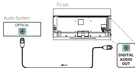
Connect the audio output of the TV labelled DIGITAL AUDIO OUT to the digital audio input of an audio system.
