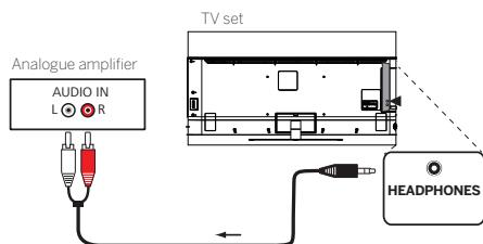
Use a stereo cinch/jack adaptor cable to connect the audio output HEADPHONES to the analogue audio input of the audio system.
