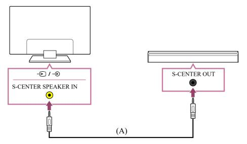
(A) TV centre speaker mode cable (supplied with sound bars that have S-CENTER OUT terminals)
