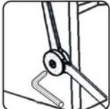
THE ACTION OF THE DOOR DAMPER CAN BE ADJUSTED WITH THE ALLEN KEY SUPPLIED. TURN CLOCKWISE TO INCREASE TENSION TO GIVE A SLOWER OPENING.
