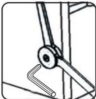
THE ACTION OF THE DOOR DAMPER CAN BE ADJUSTED WITH THE ALLEN KEY SUPPLIED. TURN CLOCKWISE TO INCREASE TENSION TO GIVE A SLOWER OPENING.
