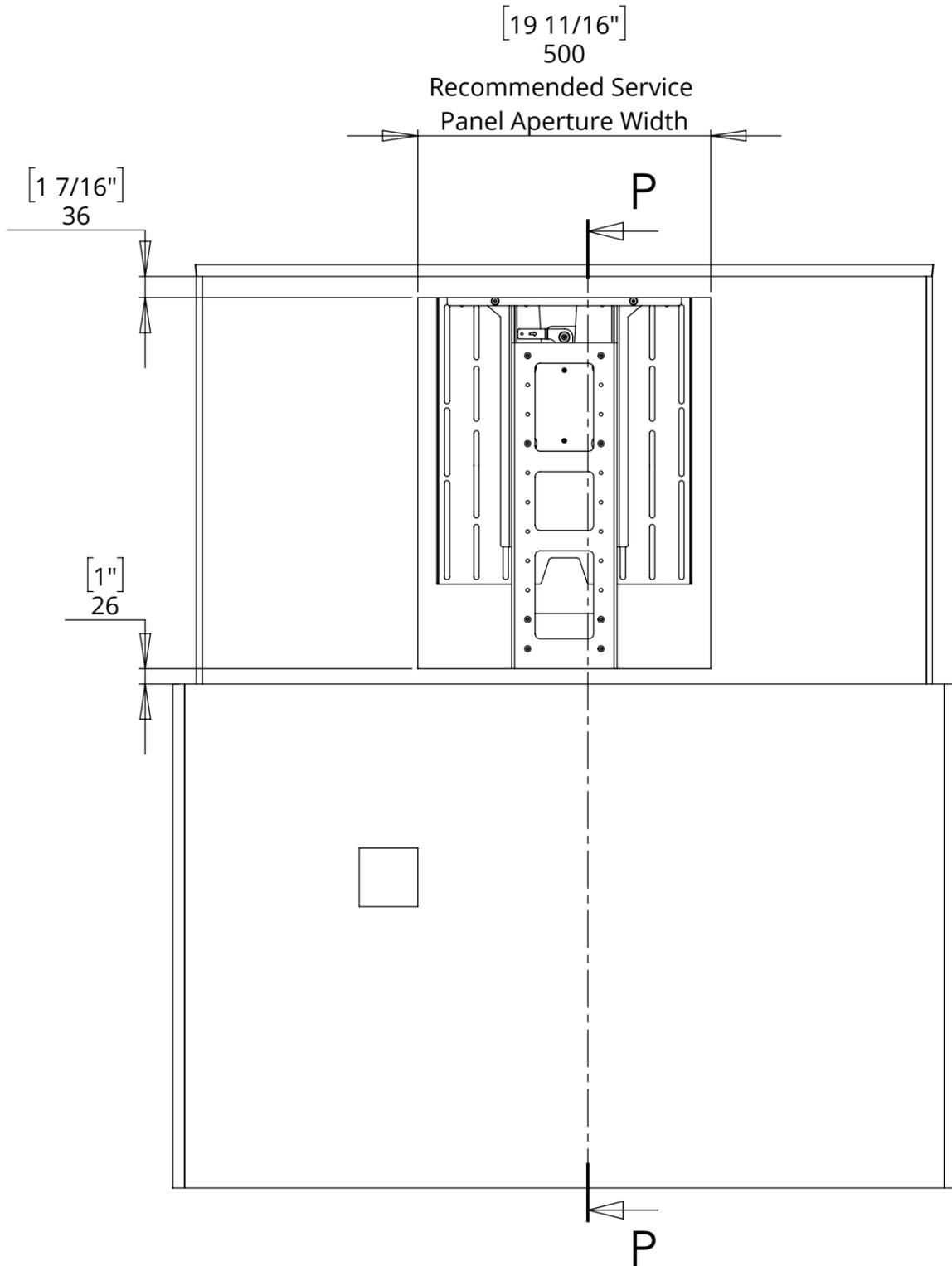
The countersink bolts enable fine tuning the position of the box enclosure relative to the uprights
