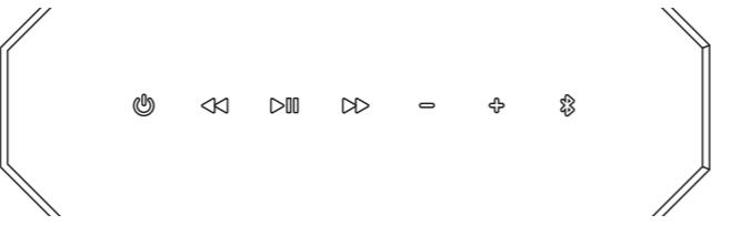
Press the power button [●] for a few seconds until the LED of the volume up button [▬▬] lights up briefly.
