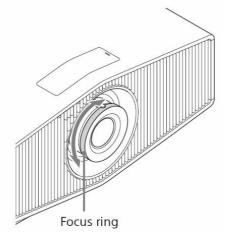
2. Adjust the focus using the focus ring
