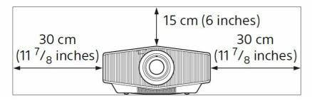
Note that the wall on the ventilation holes side may become hot. Air from air conditioners or the ventilation holes of this unit or other devices, may cause oscillation on the screen. Be sure not to install this unit in the area where the air from air conditioners or the ventilation holes of these devices reach to the front side of this unit.
