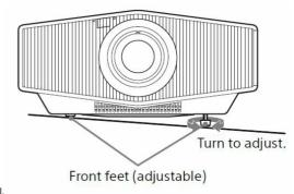
If the unit is installed on an uneven surface, use the front feet (adjustable) to keep the unit level.
