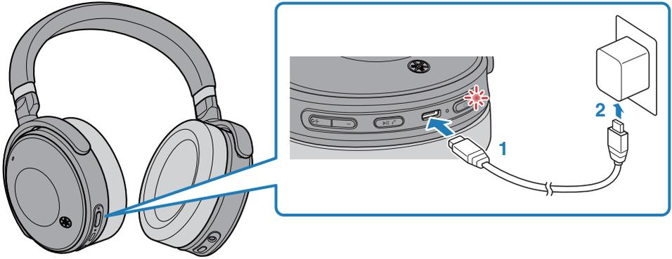
**1 Plug the USB power cable into the controller.**
