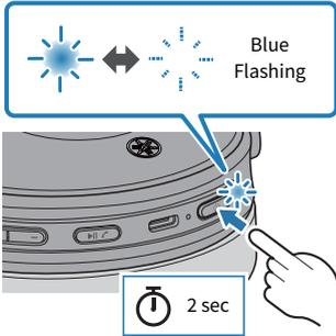
If this product do not automatically connect to a Bluetooth device, it is waiting for connection. Operate the Bluetooth device to connect with this product.
