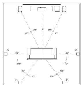
The Bronze C150 centre speaker should be positioned so that it is pointing at approximate ear height of the main listening position. Included with the Bronze C150 are 4 adhesive feet, stick these to the bottom of the cabinet for protection and to help isolate the speaker.
