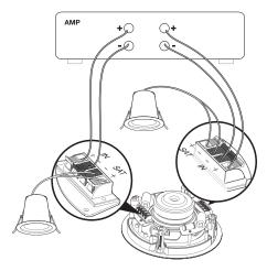
We recommend use Minx C46 Satellite speaker connect to the SAT on the C200B. The speaker cable is coded with a bead or stripe down one lead's insulation, or has differently coloured wires. Press the spring-loaded red or black tab back to reveal the connecting hole. Insert the stripped end of the speaker wire, then release the tab.
