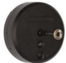
Monitor Audio's FIX-M speaker mount is designed for our middleweight speakers. FIX-M provides a strong wall mount solution, which enables speakers to be placed in a wide range of set positions and at matching angles, to ensure perfect sound dispersion. Three angles are set at 0, 15 and 30 degrees from centre, short and long insert arms are included, further increasing mounting options. The front section of the speaker mount can also be rotated,
