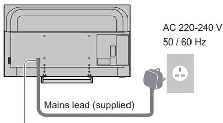
**Insert the mains plug firmly into place.**
