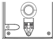
When you have installed the speaker to the wall or ceiling, then connect the speaker cable to the terminal and reinstall the front cover.
