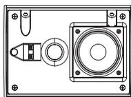
Turn the tweeter counter-clockwise to remove it from the baffle. Reinstall the new tweeter by pressing it towards the horn section of the baffle and turn it clock wise until you hear a "click".
