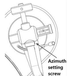
With the aid of a good magnifying glass adjust the arm tube until the needle is vertical in the groove (i.e. perpendicular to the record's surface). Ideally this should correspond to the top surface of the cartridge body being parallel to the record surface.
