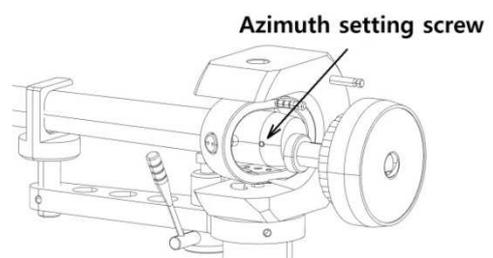
With the aid of a good magnifying glass adjust the needle until it is vertical in the groove (i.e. perpendicular to the record's surface). Ideally this should correspond to the top surface of the cartridge body being parallel to the record surface.
