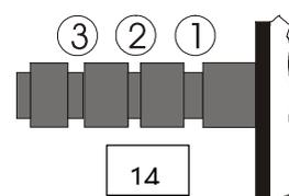
Hang the loop of the thread of the anti-skating weight in the groove of the anti-skating stub (14) corresponding to the downforce applied to your cartridge and feed the thread through the loop of the wire support (16).
