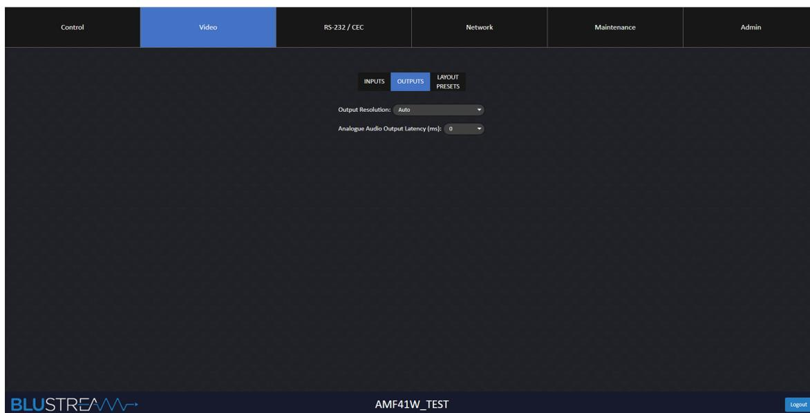
The Video Output Settings page allows a logged in user to adjust settings relating to the HDMI and analogue audio output of the AMF41W:
