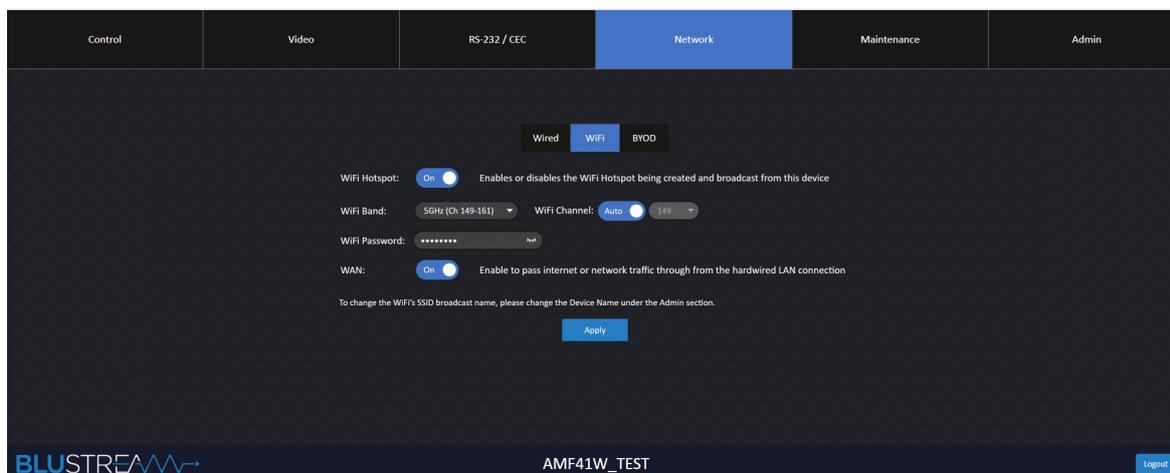
The WiFi Network Settings page allows an active user to adjust the internal WiFi hotspot settings of the AMF41W.
