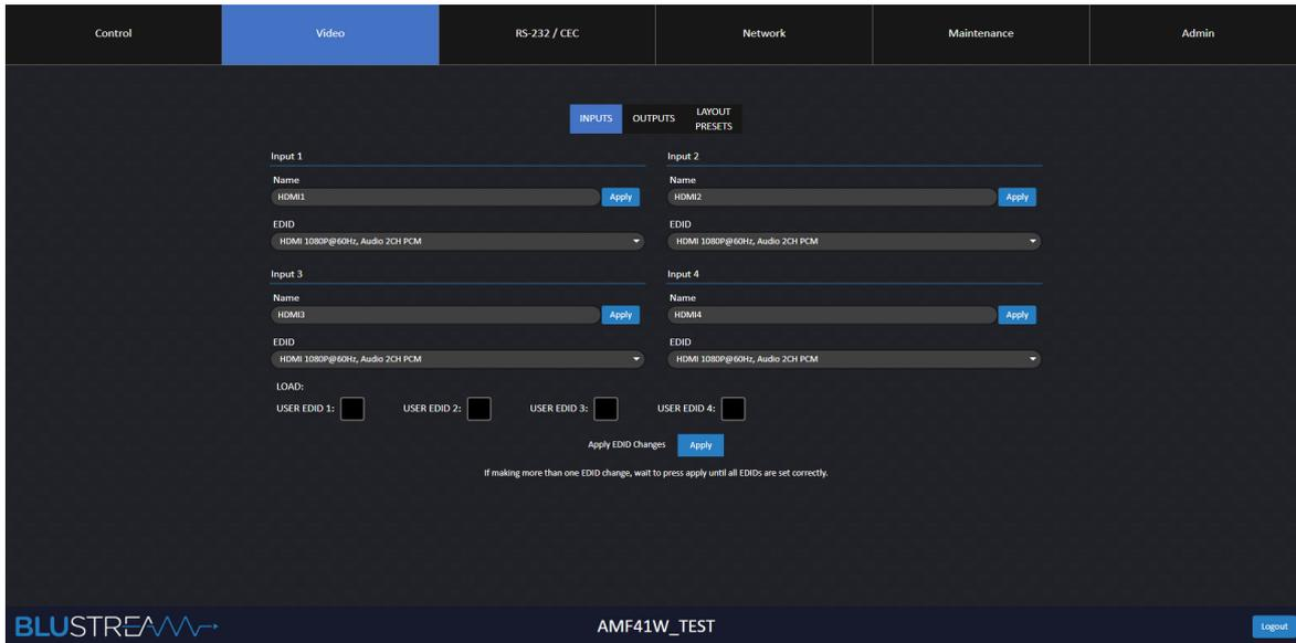
The Video Input Settings page allows a logged in user to adjust setting relating to the HDMI inputs of the AMF41W.
