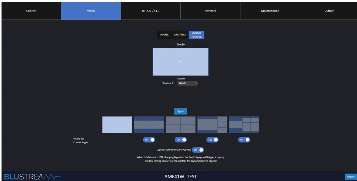
The Video Layout Presets page allows an active user to set up, and configure, the default settings for both single view and multi-view windows.
