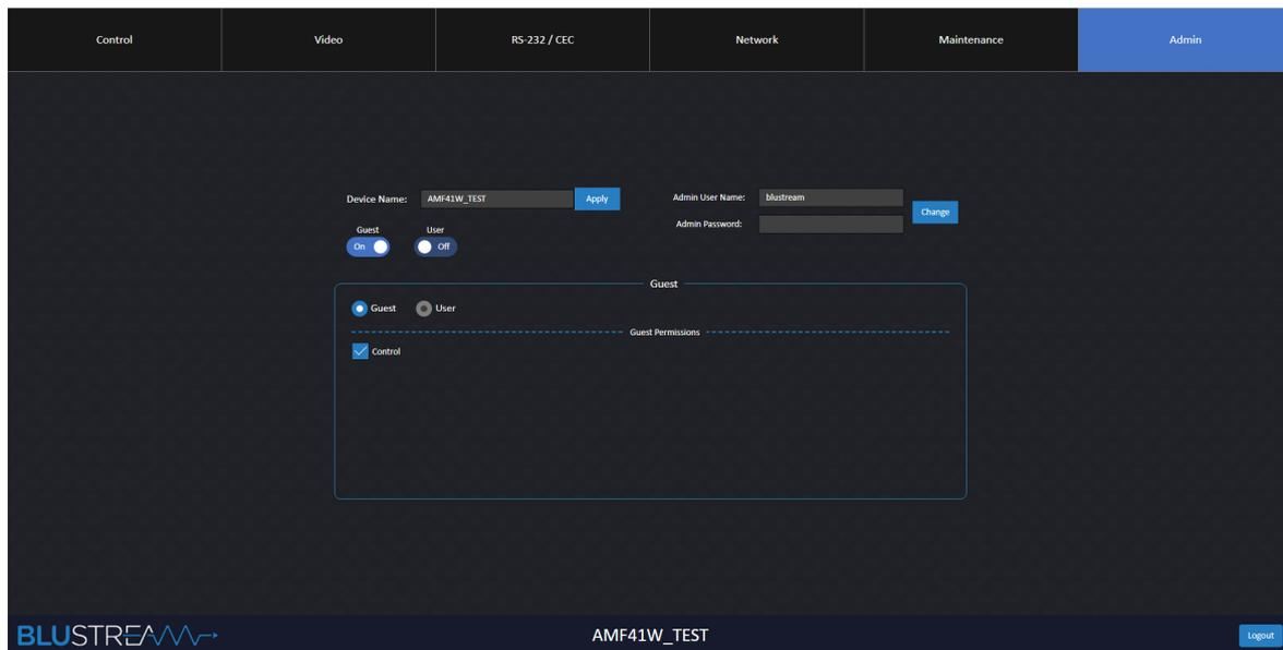
The Admin Settings page allows the admin to set up the device name or SSID of the unit, as well as enable or disable the Guest user, or special user that can be given specific privileges.
