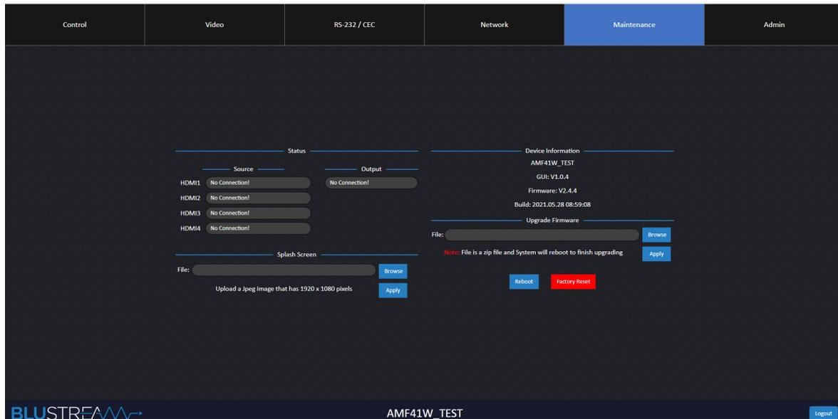
The Maintenance Settings page allows an active user to view status information about the AMF41W as well as update the splash screen or firmware of the device.
