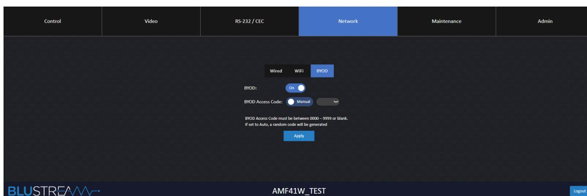
The BYOD Network Settings page allows a logged in user to adjust the BYOD settings of the AMF41W.
