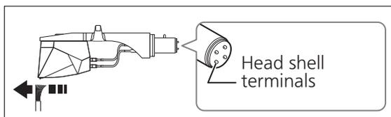
**Wipe the head shell terminals occasionally.** Wipe the head shell terminals with a soft cloth and fit the head shell to the tone arm.
