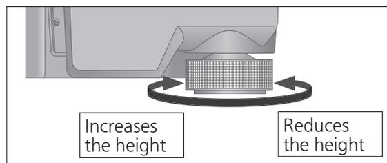
Raise the main unit to turn the insulators and adjust the height.
