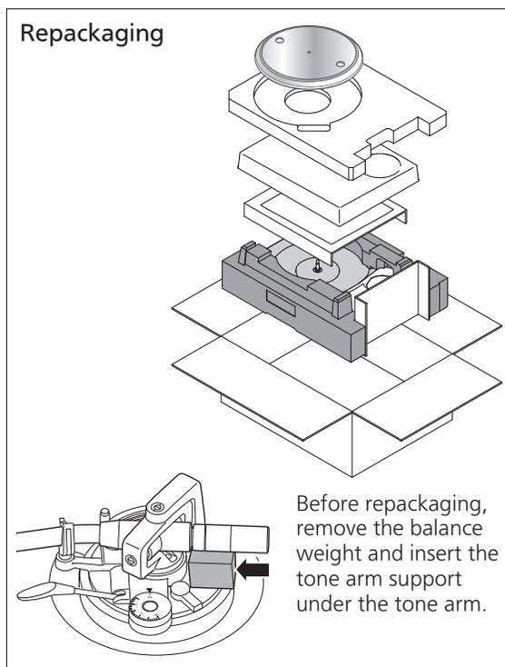
Before repackaging, remove the balance weight and insert the tone arm support under the tone arm.
