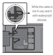
• After the cable is connected, close its cover and then tighten the loosened screws.
