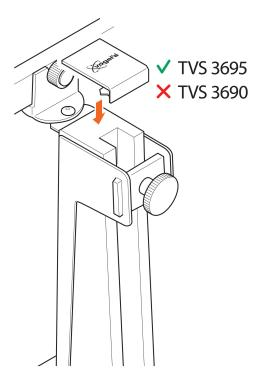
2. Apply the click-on stainless-steel **cover plate** (P) on top of the **steel bracket** (U). (TVS 3695)
