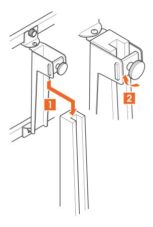
1. Slide the **steel bracket**  $\mathbb Q$  over the top of the **wooden/steel stand**  $\mathbb R$ . Use the knob (see illustration) to fasten the **steel bracket**  $\mathbb Q$  to the top of the **wooden/steel stand**  $\mathbb R$ .
