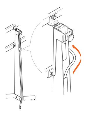
1. Carefully guide the cables through the back of the **wooden/steel stand**  ${\mathbb R}$ .
