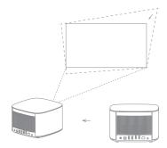
When the automatic obstacle avoidance function is enabled, the frame will automatically avoid obstacles if there are obstacles in the projection area. When the automatic screen alignment function is enabled, the frame will automatically match the screen if there is a 16:9 or 16:10 screen in the projection area.
