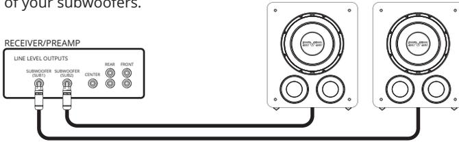
If you have more subwoofers than Sub Outputs from your AV Receiver, an easy solution is to use an RCA splitter or RCA Y-adapter to divide the subwoofer output. This is the most commonly recommended way to connect multiple subwoofers when there is only one Sub Out.
