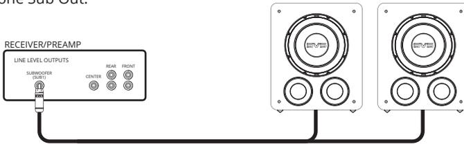
Another option is to use the Left and Right RCA outputs on the PB-1000 Pro to Daisy Chain additional subwoofers. It's important to use the matching output and input terminals. For example, if you are using the RCA inputs, be sure to use the RCA outputs to daisy chain to the next subwoofer.
