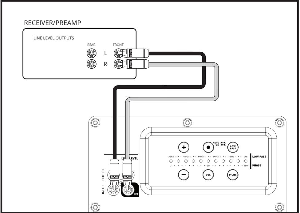
Enable and adjust the on-board low pass filter of the PB-1000 Pro for a smooth blend with the main speakers.
